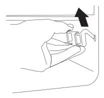
When you have finished, hook the side rails back onto the sides of the chamber. To refit the frame pull both side rails forward and equal amount. For each side in turn support the side rail and press the frame down into the side rails. Replace the grill pan.
